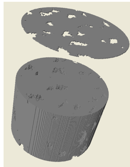
Fig. 6 Numerical pseudocore generated from training image in Figure 3 and fullbore images that correspond to Figure 1. Vugs are clear, and dense rock matrix is gray. Length of interval is 1 ft (0.3 m), and borehole diameter is 8.5 in (22 cm). The arbitrary suspended slice (top) shows that this is truly a 3D model, with throughgoing pores in every slice.
